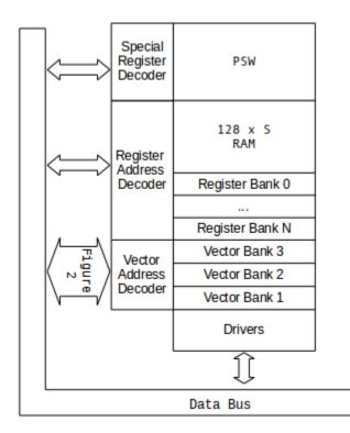
Fig. 1. Layout of the RAM with Vector Register Bank
